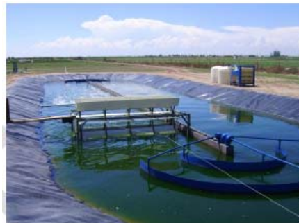
Figure 3: Microalgal production raceway in southeast New Mexico. Courtesy of the CEHMM, Carlsbad, NM, www.cehmm.org
