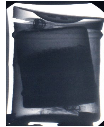
Breached nuclear waste container due to plutonium reaction
