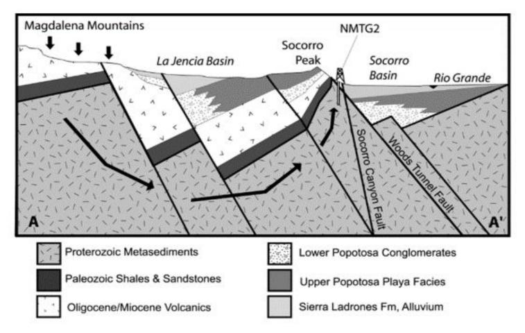
Precipitation percolates into the subsurface, where it is heated by elevated temperatures associated with the Rio Grande rift extension. Heated groundwater moves back up to the surface along rift-related faults.
