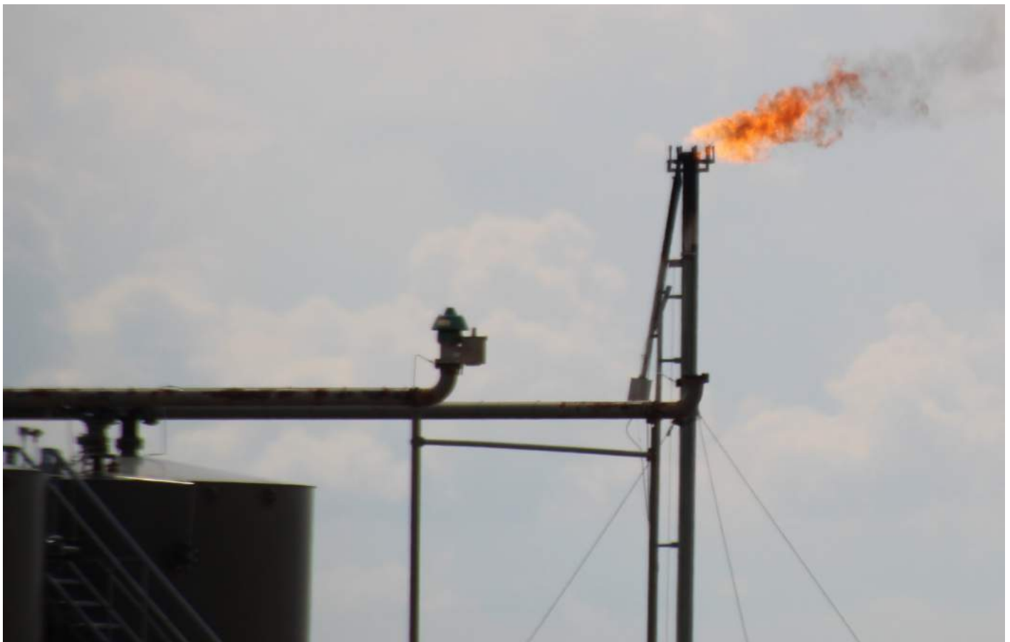
A poorly lit flare at Rustler Breaks SWD #6/ API #30-015-45034, a San Mateo Midstream facility in Eddy County, New Mexico, Sept. 2022. Photo credit Charlie Barrett, Earthworks.
